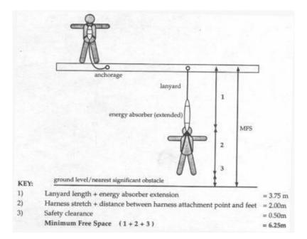
Before use, harnesses, fall arresters and tank rescue belts must be visually inspected by the user, and inspected annually by an independent institute. A record must be kept of this. They must be replaced immediately once they have withstood a strain.
